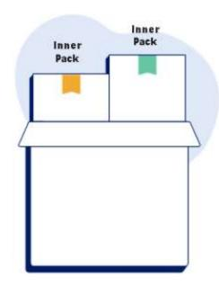
If contents < 23kg. (50 lbs.), must use double-wall corrugation. If contents < 31kg. (68 lbs.), must use triple-wall corrugation. Must score a minimum 90 kg (200 lb.). on the bursting strength\* test and 32 on the edge crush test\*.
