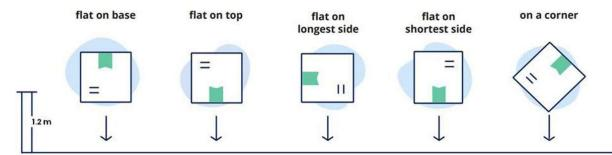
If your packaging can protect your product during these tests, it has passed the 4-foot drop test. Products must also withstand a full-minute vigorous shaking test without any of the contents breaking.
