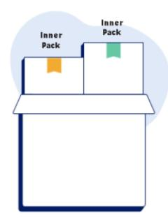
If contents < 23kg. (50 lbs.), must use double-wall corrugation. If contents < 31kg. (68 lbs.), must use triple-wall corrugation. Must score a minimum 90 kg (200 lb.). on the bursting strength\* test and 32 on the edge crush test\*.
